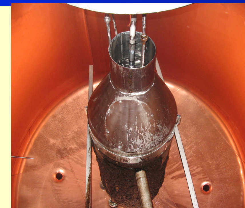
Figure 4 Kettle after caustic/peroxide wash
